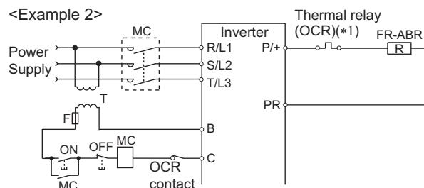
\*1 Refer to the following table for the thermal relay models for each capacity. Refer to the following diagram for connection. (Always install a thermal relay when using a brake resistor for the inverters with 11K or higher capacity.)
