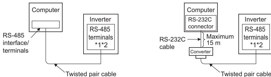
\*1 Set the terminating resistor switch (SW4) to the  $100\ \Omega$  side.
