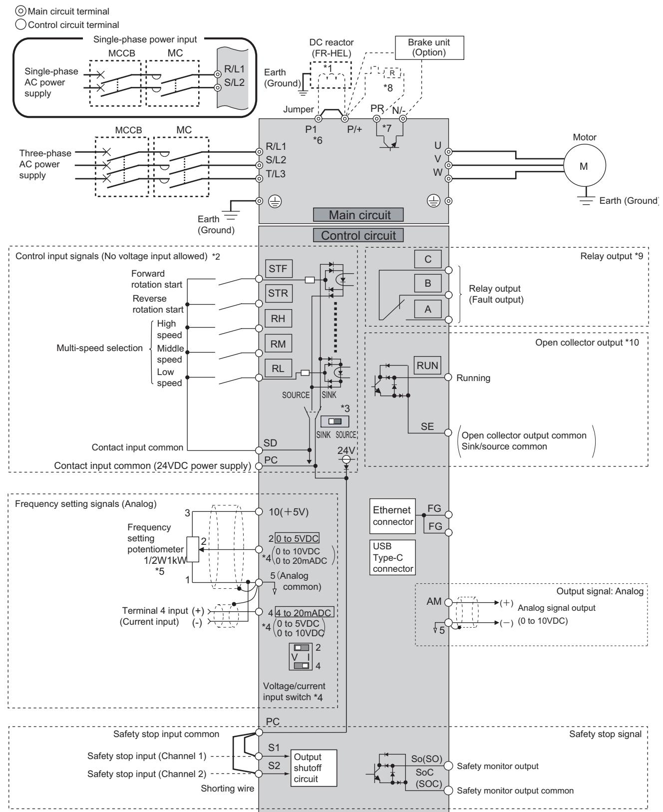
\*1 Remove the jumper between P1 and P/+ to connect the DC reactor. (Single-phase 100 V power input model is not compatible with the DC reactor.)
