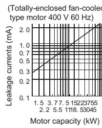
For "Y" connection, the amount of leakage current is approx. 1/3 of the above value.
