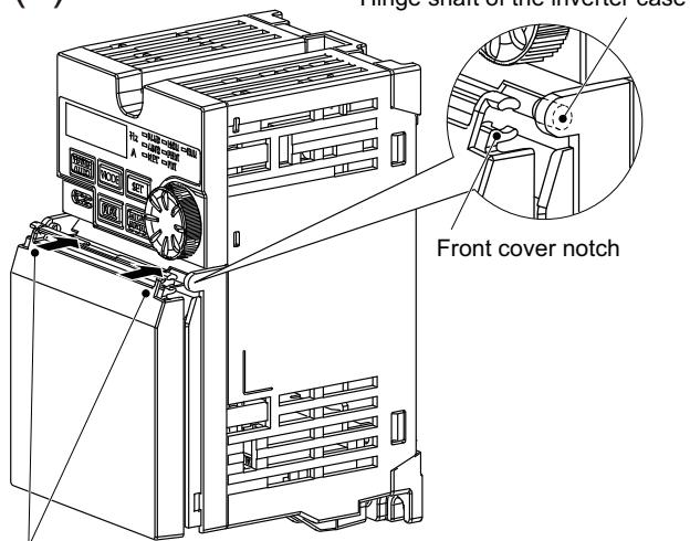
Push the upper corners of the front cover, and snap the notches onto the hinge shaft of the inverter case.
