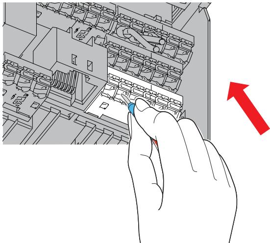
When using single wire or stranded wire without crimp terminal, push the open/close button all the way down with a flathead screw driver, and insert the wire.
