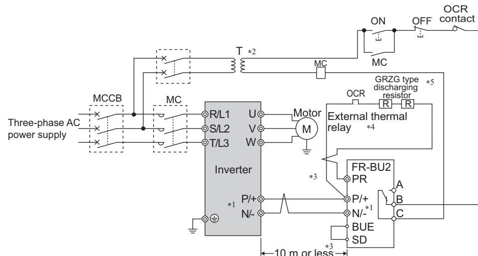
\*1 When wiring, make sure to match the terminal symbols (P/+ , N/-) on the inverter and on the brake unit (FR-BU2). (Incorrect connection will damage the inverter and brake unit.)
