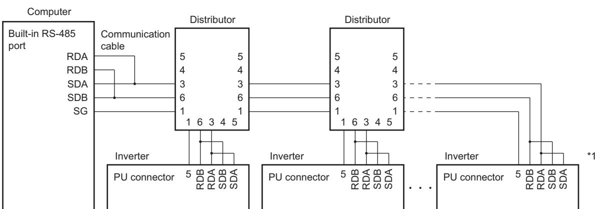
\*1 On the inverter most remotely connected with the computer, set the terminating resistor switch (SW4) to the 100 Ω side.
