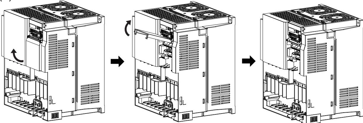
(a) With the terminal block cover removed, pull open the front cover 90° or more to remove it from the hinge shaft of the inverter case.
