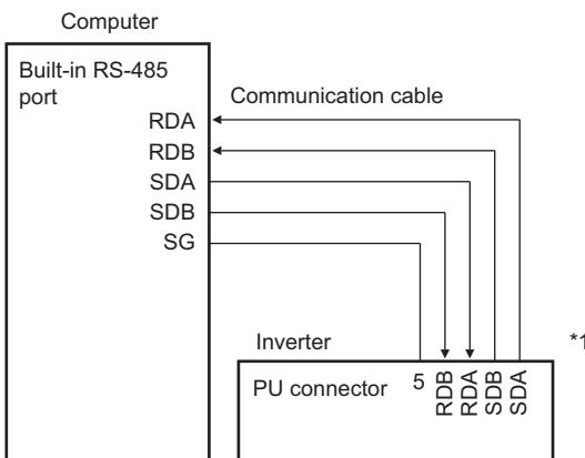
\*1 Set the terminating resistor switch (SW4) to the 100 Ω side.
