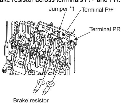
Diagram showing a terminal block with a jumper wire connected between terminals P/+ and PR. A brake resistor is connected in parallel across these terminals. Labels include Jumper \*1, Terminal P/+, Terminal PR, and Brake resistor.
