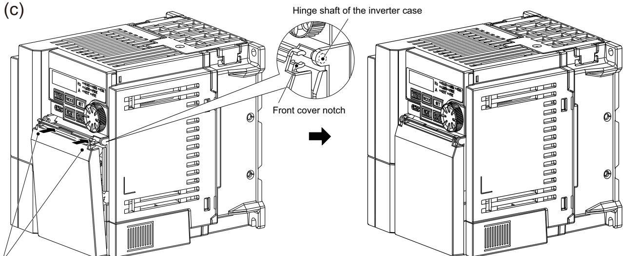
Push the upper corners of the front cover, and snap the notches onto the hinge shaft of the inverter case.
