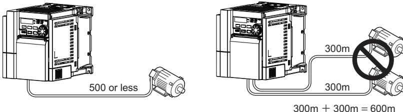
When driving a 400 V class motor by the inverter, surge voltages attributable to the wiring constants may occur at the motor terminals, deteriorating the insulation of the motor. In this case, take one of the following measure.
