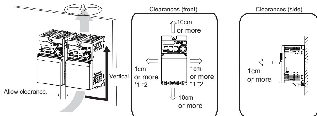
\*1 When using the inverters at the surrounding air temperature of 40°C or less, the inverters can be installed side-by-side (closely attached with 0 cm clearance).
