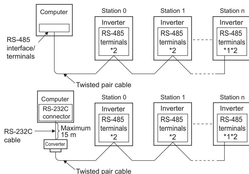
\*1 On the inverter most remotely connected with the computer, set the terminating resistor switch (SW4) to the  $100\ \Omega$  side.
