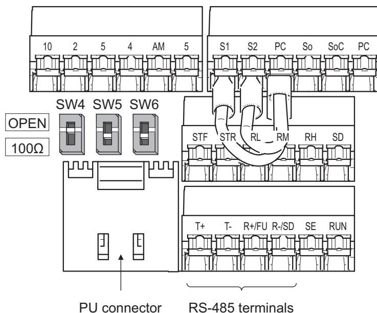
1. If any cable is connected to the PU connector, remove the wiring.
