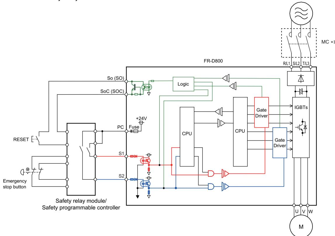
\*1 To avoid an electric shock hazard during wiring or inspection, install a magnetic contactor (MC) at the input side of the inverter.
