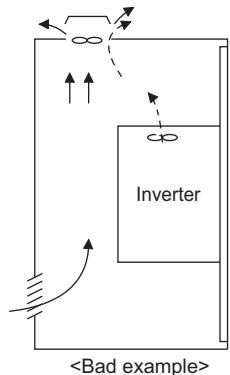
Arrangement of the ventilation fan and inverter
