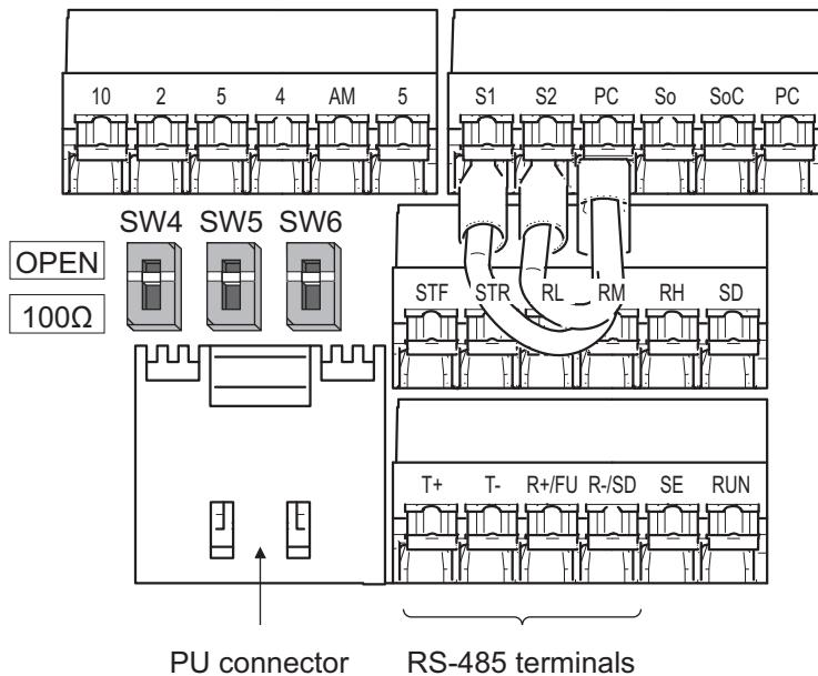
1. If any cable is connected to the RS-485 terminals, remove the wiring.
