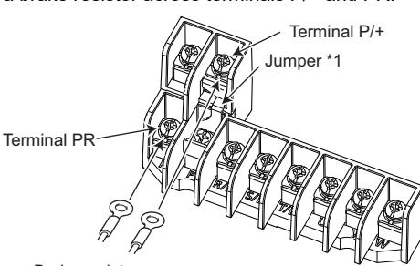
Diagram showing a terminal block with a jumper wire connected between terminals P/+ and PR. A brake resistor is connected in parallel across these terminals. Labels include Terminal P/+, Jumper \*1, Terminal PR, and Brake resistor.
