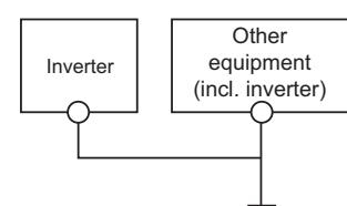
(I) Separate earthing (grounding): Good    (II) Common (single-point) earthing (grounding): OK    (III) Inadequate common (single-point) earthing (grounding): Bad
