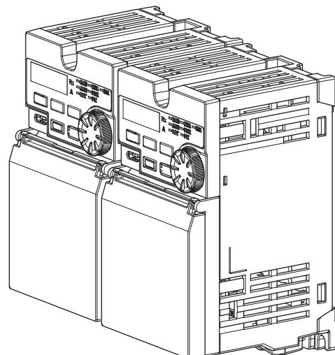
(a) Push the front cover downward using its upper end as a support to close the cover.
