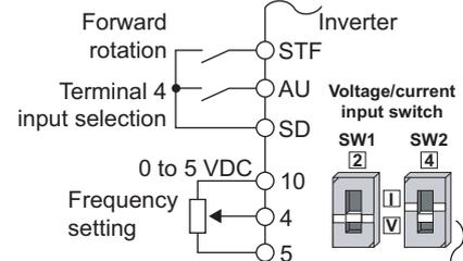
Connection diagram using terminal 4 (0 to 5 VDC)
