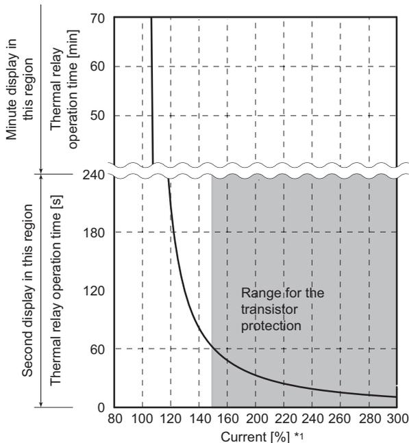
Protective function activated area: the area right of the characteristic curve
