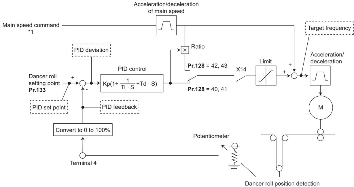
\*1 The main speed can be selected in all operation modes, External (analog voltage input, multi-speed), PU (digital frequency setting) and Communication.
