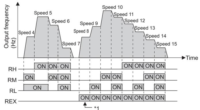
\*1 When the RH, RM and RL signals are OFF and the REX signal is ON while "9999" is set to **Pr.232 Multi-speed setting (speed 8)**, the inverter operates at the frequency set in **Pr.6**.
