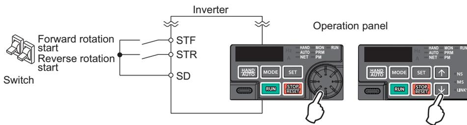
The following shows the procedure to operate at 30 Hz.
