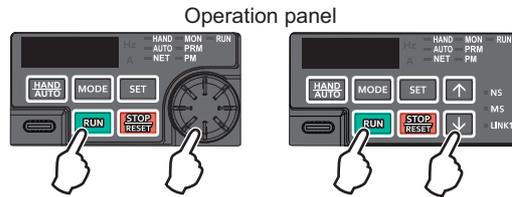
The following shows the procedure to operate at 30 Hz.
