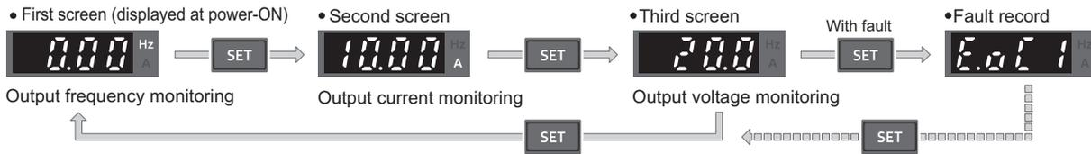
The following is the screen flow diagram when **Pr.52** = "20" (cumulative energization time).
