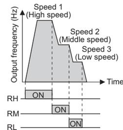
The following shows the procedure to operate at a high speed (60 Hz).
