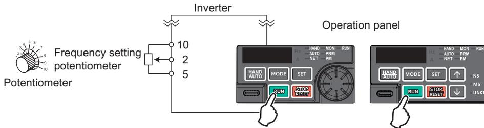
The following shows the procedure to operate at 60 Hz.
