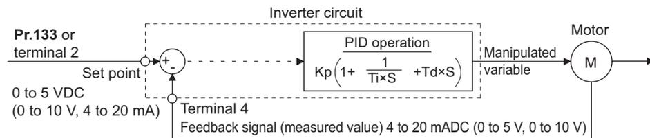
Kp: Proportionality constant Ti: Integral time S: Operator Td: Differential time
