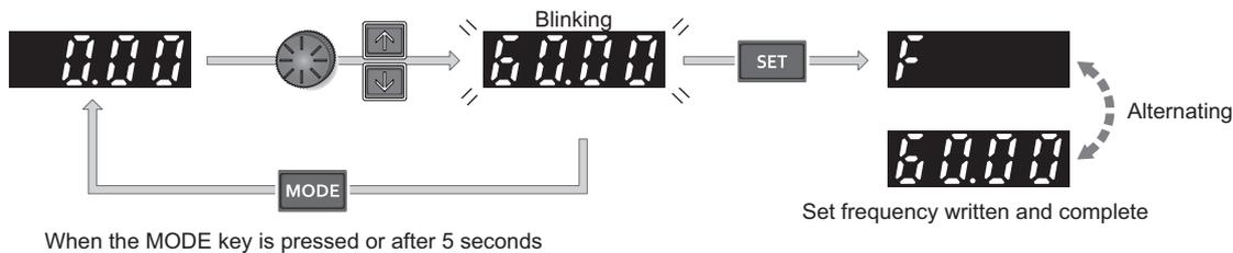
When the automatic frequency setting is enabled (Pr.161 = "1 or 11")
