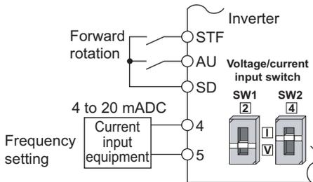
Connection diagram using terminal 4 (4 to 20 mADC)
