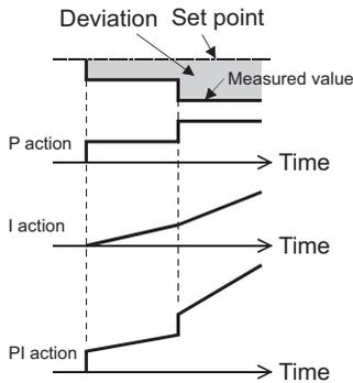
(Note) PI action is the result of P and I actions being added together.
