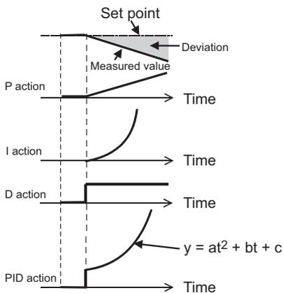
(Note) PID action is the result of all P, I, and D actions being added together.
