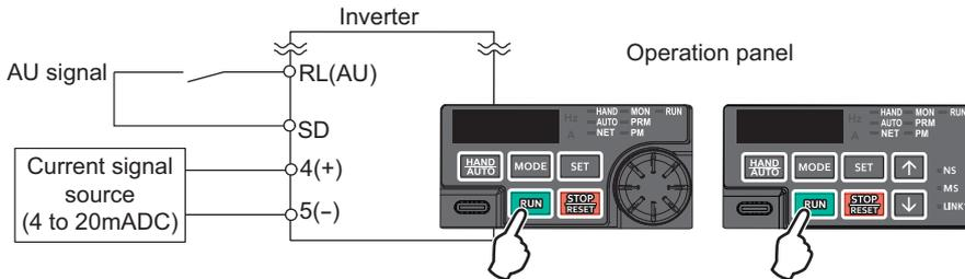
The following shows the procedure to operate at 60 Hz.
