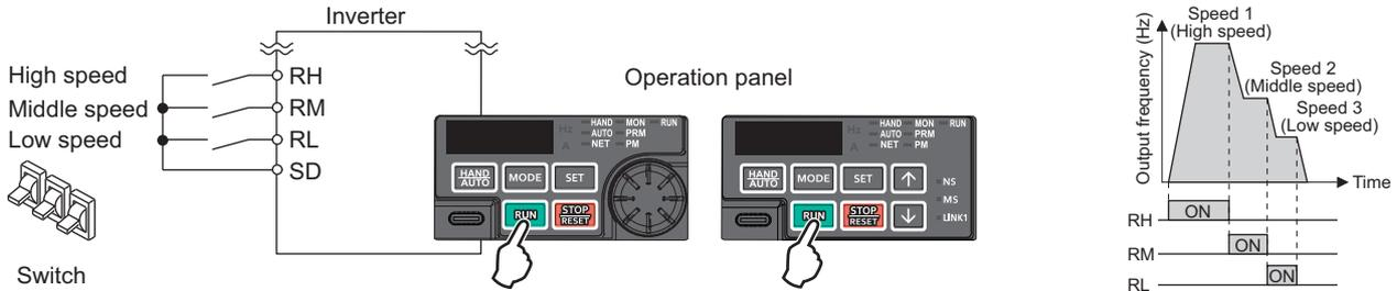
The following shows the procedure to operate at a low speed (10 Hz).
