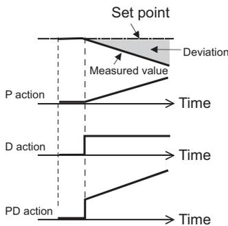
(Note) PD action is the result of P and D actions being added together.
