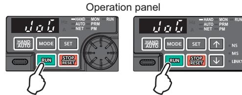
The following shows the procedure to operate at 5 Hz.
