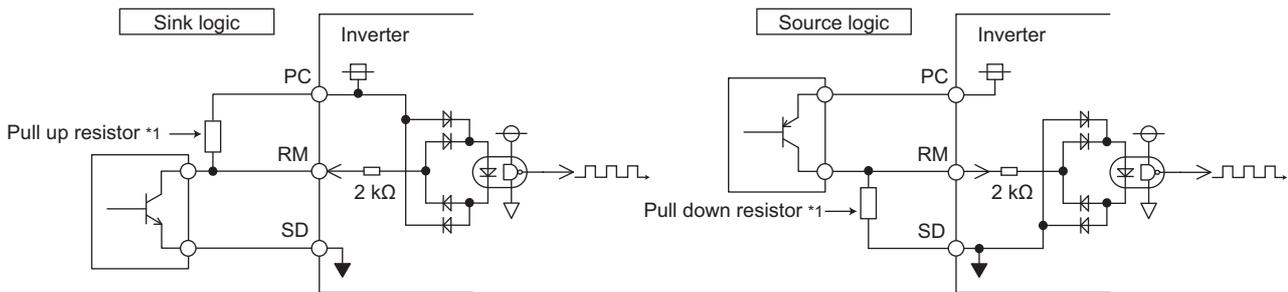
\*1 When the wiring length is long with open collector outputs, the influence of stray capacitance causes the pulse to flatten out and prevents the input pulse from being recognized.
