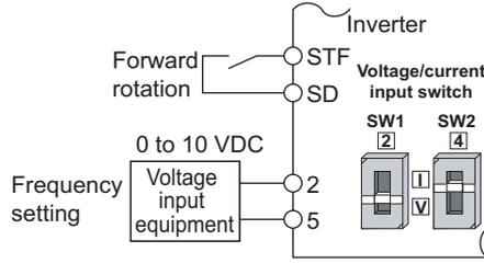
Connection diagram using terminal 2 (0 to 10 VDC)
