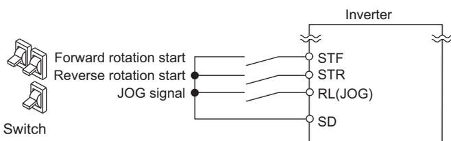
The following shows the procedure to operate at 5 Hz.
