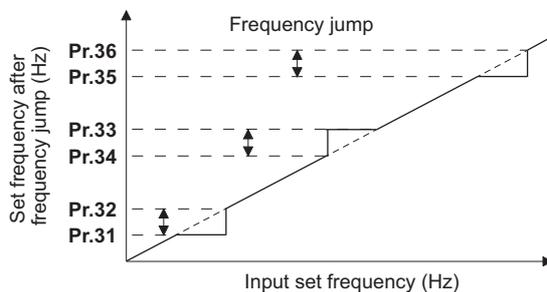
Example 1) To fix the frequency to 30 Hz in the range of 30 Hz to 35 Hz, set 35 Hz in **Pr.34** and 30 Hz in **Pr.33**.
