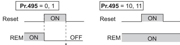
\* When **Pr.495** = "1", the signal condition saved in EEPROM (condition of the last power OFF) is applied.
