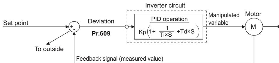
Kp: Proportionality constant Ti: Integral time S: Operator Td: Differential time
