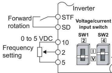
Connection diagram using terminal 2 (0 to 5 VDC)
