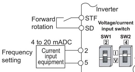
Connection diagram using terminal 2 (4 to 20 mADC)
