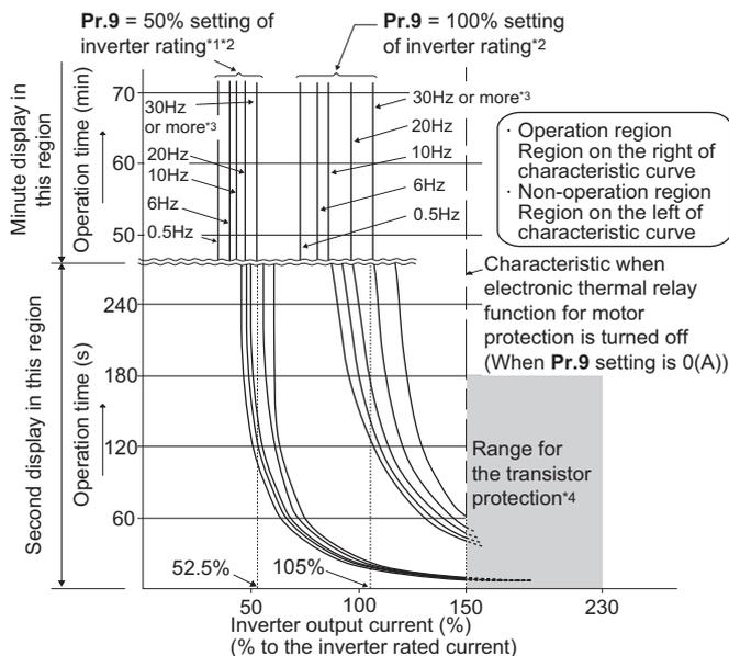
\*1 When setting **Pr.9** to a value (current value) of 50% of the inverter rated current
