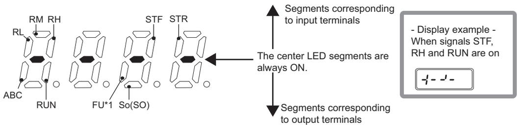
\*1 Monitoring is available only for the standard model. The status of terminal FU is displayed regardless of the R/FU switch (SW5) setting.
