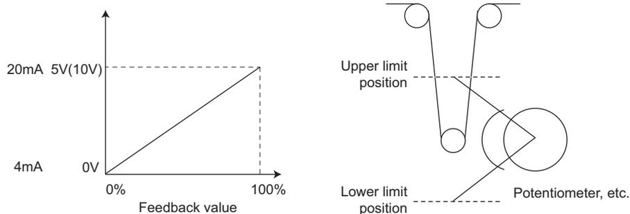
(Example) To execute control at the dancer center position using a 0 to 7 V potentiometer
