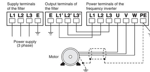
All cables must be shielded and earthed at both ends in order to reduce cable radiation. Earth motor, bond to filters. For environmental conditions and mounting position please note the instructions in the operation manual for the frequency inverter FR-E700 EC.
