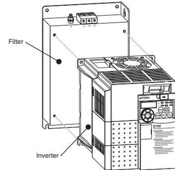
To fix the filter-inverter unit on the back of the cabinet use the mounting bolts provided with the filter. For correct filter performance the filter mounting bolts should electrically bond to the cabinet back panel which is connected to earth. If this is not possible, the paint should be removed from the cabinet directly under the filter footprint.
