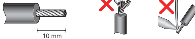
Cable sheath stripping length
