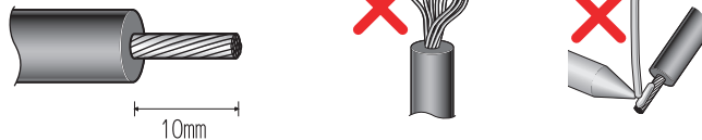
Cable sheath stripping length
